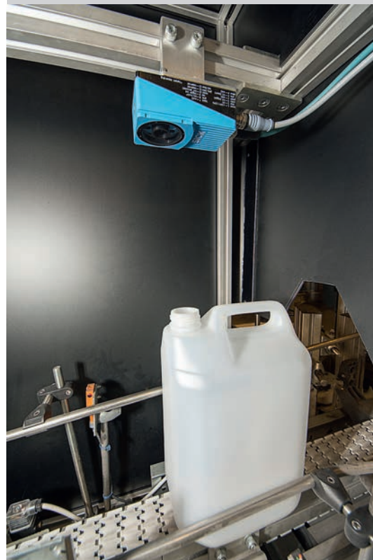
Inspection for defects in bottle neck
