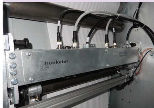
Web inspection using Mitsubishi Electric Line Scan Bar (Courtesy Hunkeler)
