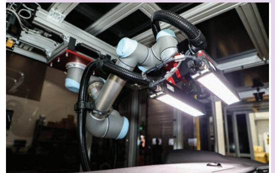
IVS Robot inspection
