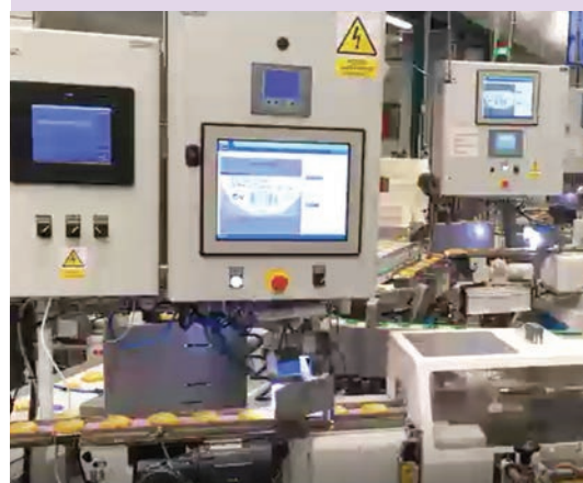
LabelChecker inspecting chocolates
