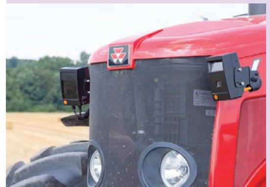
3D sensors mounted on tractor
