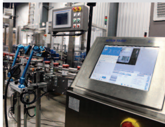
CI-Vision inspection system at Crofter's Foods (courtesy Canadian Packaging)
